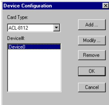
To modify the settings of IRQ level, DMA channel and Base Address of a device, click “Modify...” button and a *Driver Configuration* window appears for you to modify DMA channel, IRQ level and base address.
