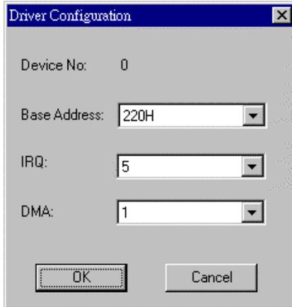
Inside the Base Address, DMA and IRQ fields are the originally set values. Modify the values and then click “OK” button. The settings for the device will be changed as you modified and return to *Device Configuration* window. Then you can click ‘OK” button in *Device Configuration* window and the settings for the driver will be modified.
