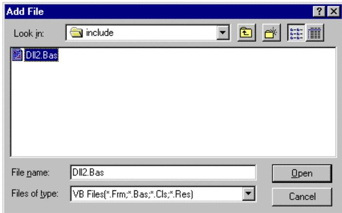
Select DLL2.BAS from the Files list by double clicking on it. If you can't find this file in the list, make sure the list is displaying files from the correct directory. By default, DLL2.BAS is installed in C:\ACL-DLL2\INCLUDE.
