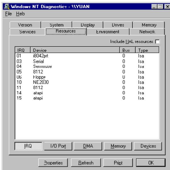
Each button in this window links to the corresponding hardware information. Therefore you can get the resource allocation information in your system and check if your DLL2 devices are loaded successfully. Please refer to Windows NT user's manual for the details about this program. The resource setting modification of DLL2 devices is described in following section.
