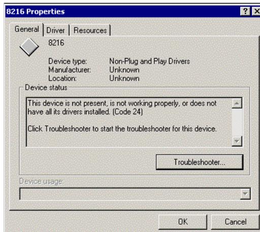
To solve this problem, you can *right-click* the device icon, and select the **Scan for hardware changes** item in pop-up menu. The system will re-load the device drivers with the resource registered in system registry.
