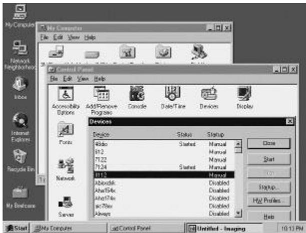
If the device status is none, you have to select the 6126, 8111, 8112, 8216, 8316 or Dio device and press the **Start** button.
