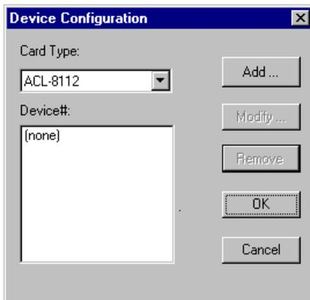
From this window you can select the driver you want to register. Since Dll2 drivers for Windows NT/2000 can support more than one device, you can configure more than one device for each
