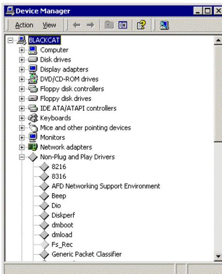
And then you can double-click the device and select the **Resources** tab to check if I/O port and IRQ resources for the device are allocated successfully.
