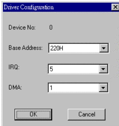
After the setting for DMA channel, IRQ level and base address, click **OK** and *Device Configuration* window re-appears. The device you just added is shown on “Device#” list as the following figure.
