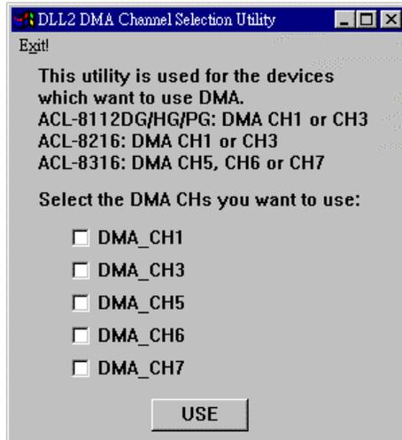
Check the desired DMA channels and then click **USE** button to inform the system that the DMA channels the DLL2 devices will use. Then you select **Exit!** command in the menu bar to exit *DLL2 DMA Channel Selection Utility*. Re-start Windows 95/98 system to make the system DMA channels selection effective.
